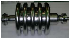
Fig. 1. Prototype five-cell cavity
