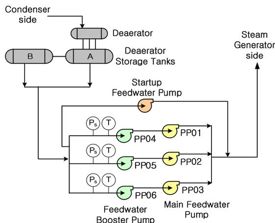
Fig. 1. Schematic diagram of SKN 1 feedwater system.
