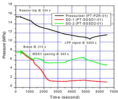
Fig. 2 Pressure trend at the pressurizer and SG dome
