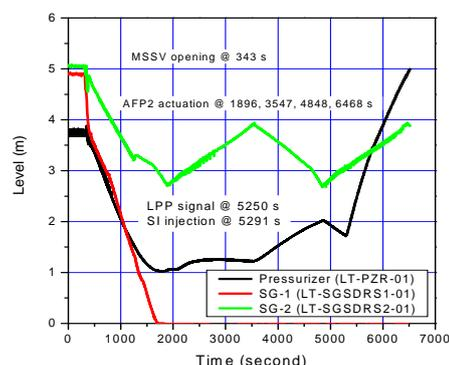
Fig. 3 Collapsed water levels in the pressurizer and the SG secondary side
