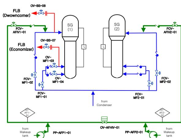
Fig. 1 Piping arrangement of feedwater line break
