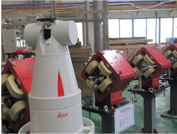
Figure 3. The fiducialization of the quadrupole magnet by using the laser tracker.
