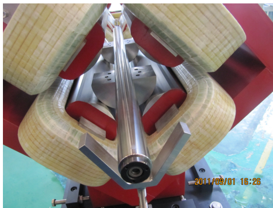
Figure 2. A mandrel and a pair of sleeves for the measurement of mechanical center.
