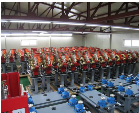
Figure 1. Magnets for the PEFP beamlines including 2 AC magnets, 107 Quadrupole magnets and 11 Bending magnets.
