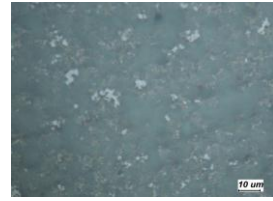
Fig. 6. SiC-coated sample exposed to the cavitation flow
