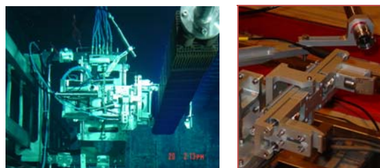
Fig. 1. Setup of LVDT for Grid Width Measurement
