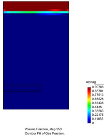
Fig.4. Gas void fraction at  $t=950$ .
