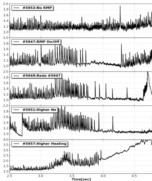
Fig. 2. ELM suppression and mitigation by applying RMP during H-mode phase. The spikes of H-alpha line corresponds to each ELM burst.
