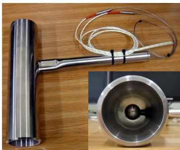
Fig. 5. The fabricated transducer of low flow meter in KAERI.
