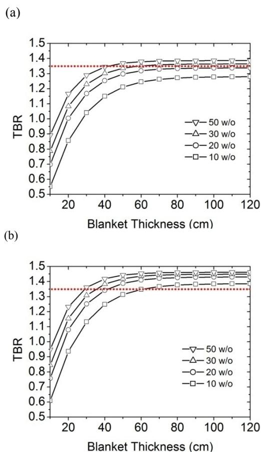
FIG. 1. TBR as a function of outboard blanket thickness when  $A = 1.5$  with inboard shield material (a) WC and (b) WC-Pb (20 cm thick Pb layer added to the WC shield).
