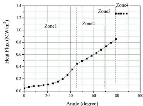
Fig. 3 Heat flux on the reactor inner wall.
