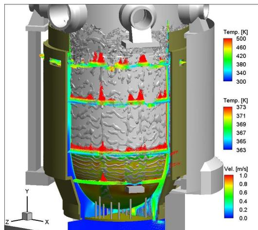
Fig. 4 Bubble behavior, velocity vectors and temperature distributions on the outer surface of the vessel and cooling water ( $T_{water} = 90^{\circ}C$ ).
