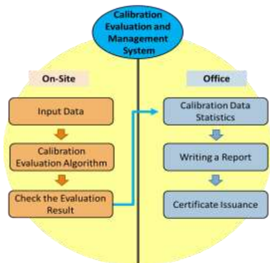
Figure 1. Calibration Evaluation and Management System Schematic
