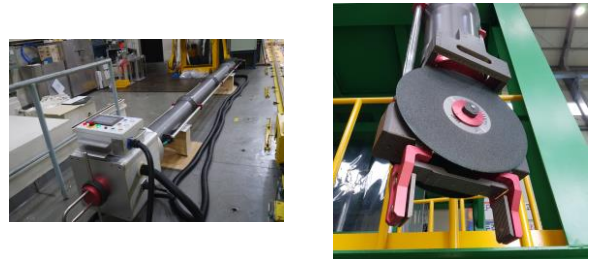
Figure 1. Underwater cutting equipment for spent nuclear fuel skeleton
