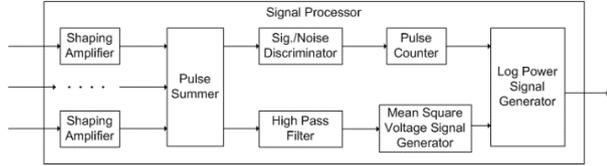
Figure 1. Signal processing diagram for logarithmic power signal
