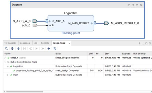
Figure 2. Hardware resource for logarithm function block
