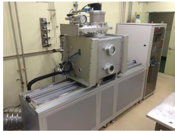
Fig. 1. Custom Physical Vapor Deposition (PVD) System Developed for Coating U-Mo Powder.
