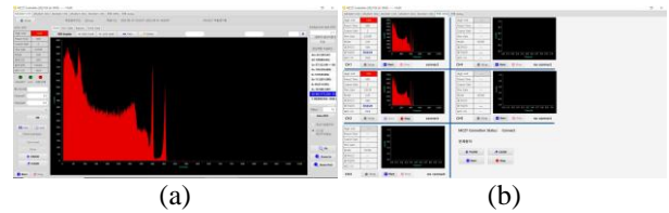
Fig. 1. Software measurement screen: (a) single-channel CZT sensor for detail analysis, (b) multi-channel CZT sensors for simultaneous monitoring.
