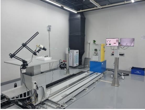
Fig. 1. CsI(Tl) detector and gamma-ray irradiator at the Radiation Device Test Center of the Korea Association for Radiation Application(KARA).
