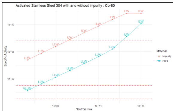
Figure 3. Co-60 specific activity of activated SS304 waste by neutron flux.
