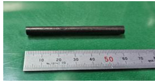
Fig. 3. Fabricated annular fuel using mold #3.
