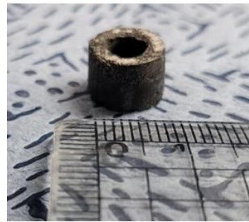
Fig. 1. Annular U-10Zr fuel pellet fabricated by cold sintering.
