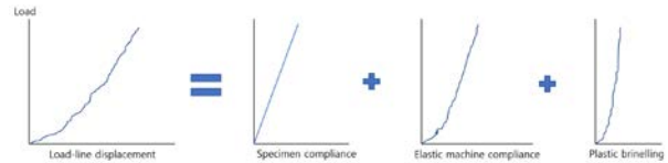
Fig. 1. Constituents of deflections in specimen and test system.
