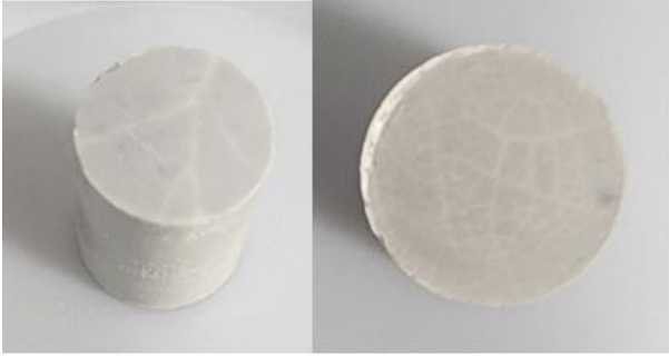
Fig. 3. Quenched \text{CeO}_2\text{-Gd}_2\text{O}_3 CSBA pellets
