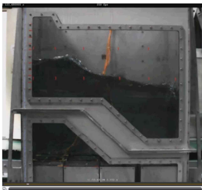
Fig. 2. Sloshing simulation tests on a small model of SFSP
