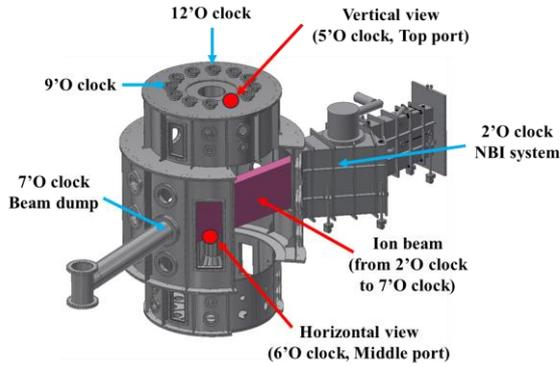
Fig. 1. Cross sectional view of VEST with NBI system. Ion beam trajectory is represented as pink block inside the chamber. Blue arrows denote direction of ports of VEST. Ports in VEST are named in clockwise order. The red dots indicate the horizontal and vertical measurement points.
