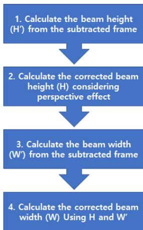
Fig. 4. Flow chart for correcting beam height and width obtained from each subtracted frame.
