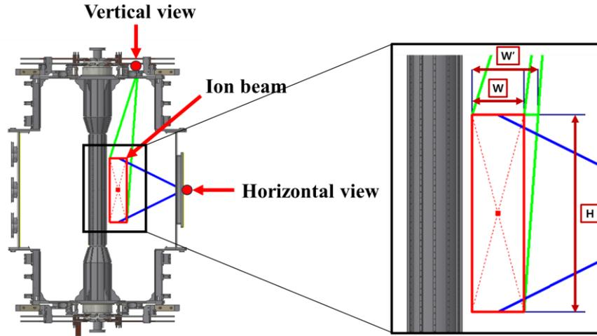
Fig. 6. Vertical cross-sectional view of VEST and magnified view to denote parameters to calculate corrected beam width. ( $W$  is corrected beam width,  $W'$  is beam width calculated from raw subtracted frame,  $H$  is corrected beam height and  $H'$  is beam height calculated from raw subtracted frame)
