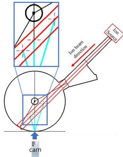
Fig. 5. Schematic top view of VEST chamber. The red lines denote ion beam. The cyan lines indicate the horizontal view itself and distance from the center of the beam to camera, which should be considered when calculating the beam height.
