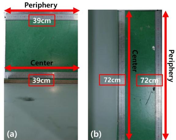
Fig. 2. Test images for checking camera distortion between center and periphery (a) Vertically (b) Horizontally.
