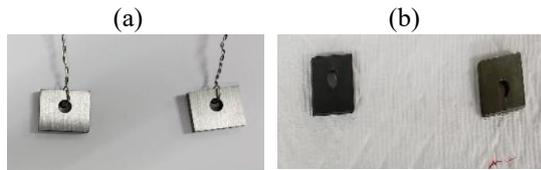
Fig. 1. Carbon Steel (CS) coupon (a) before, and (b) after dissolution reaction, left 10 mM, right 20 mM.
