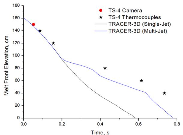
Fig. 6. Jet front elevation in TS-4 simulation
