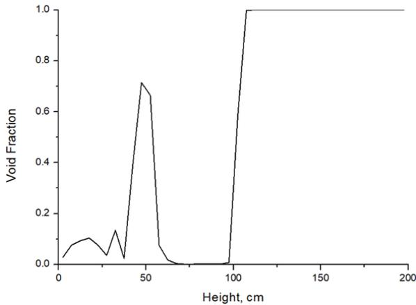
Fig. 7. Axial void fraction distribution at the time of triggering in TS-4 simulation
