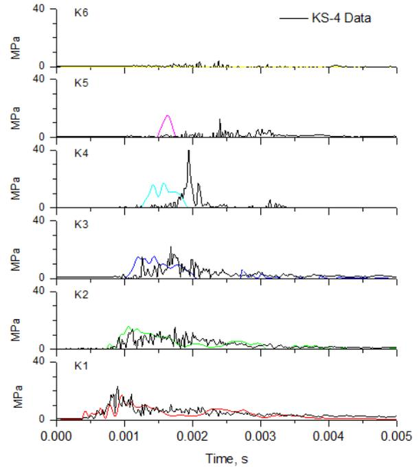
Fig. 5. Explosion pressure traces in KS-4 simulation
