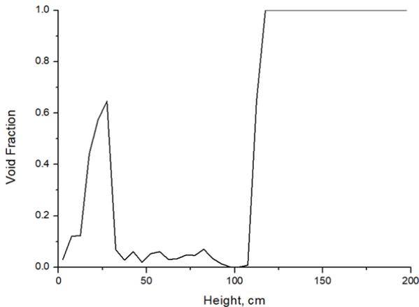
Fig. 4. Axial void fraction distribution at the time of triggering in KS-4 simulation
