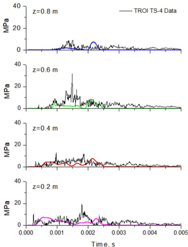
Fig. 8. Explosion pressure traces in TS-4 simulation
