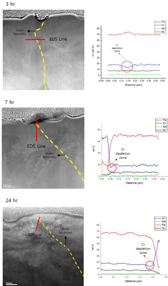
Fig. 12. STEM image and EDS (wt.%) for Cr carbide in heat treatment sample
