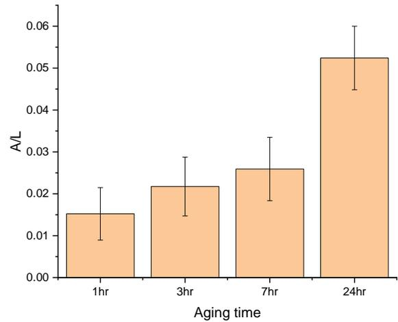
Fig. 7. Cr carbide area per grain boundary by heat treatment time
