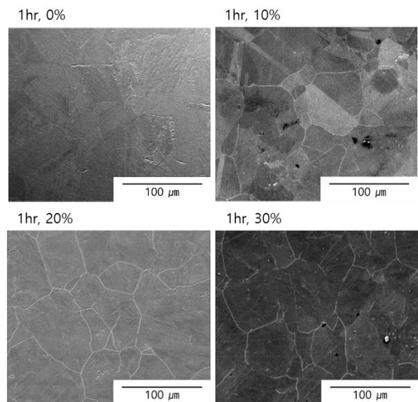
Fig. 9. SEM images for reduction rate
