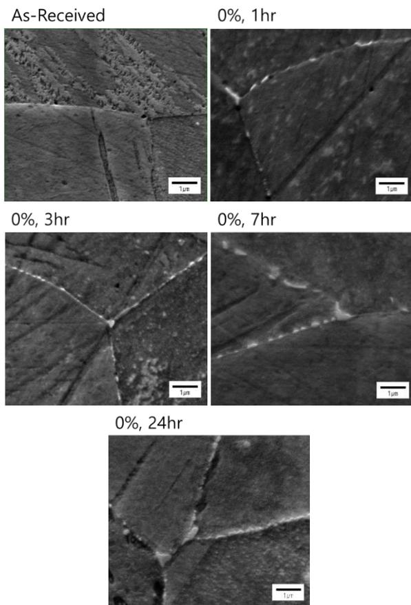
Fig. 6. Microstructure by heat treatment time
