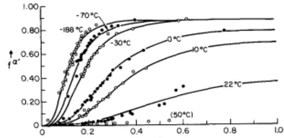
Fig. 3. Martensite fraction by temperature for stainless 304 [3]
