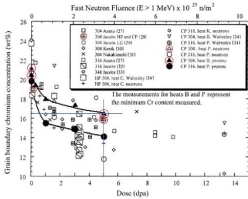
Fig. 13. Cr composition as a function of dose for irradiated [5]
