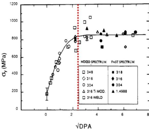
Fig. 14. Yield strength for neutron irradiation dose [7]
