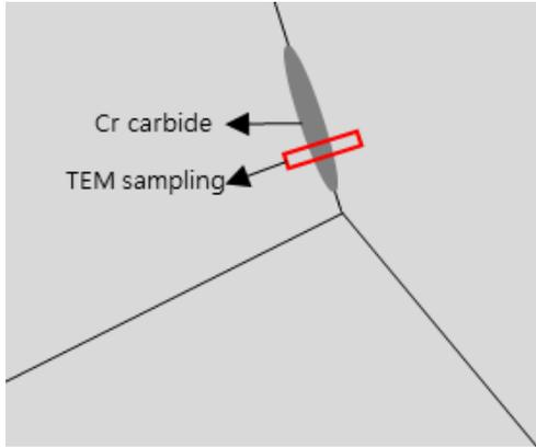
Fig. 10. TEM Sample cutting method
