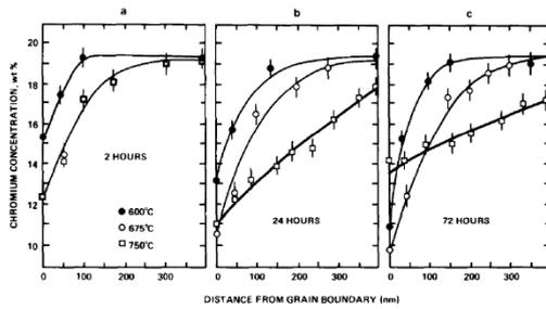
Fig. 2. Chromium concentration profiles obtained from specimens sensitized of (a) 2h, (b) 24h, and (c) 72h at 600°C, 675°C and 750°C [2]
