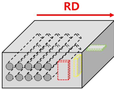
Fig. 5. Rolling direction and specimen direction
