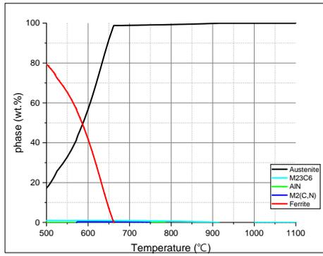
Fig. 1. Phase diagram of Stainless steel 304H
