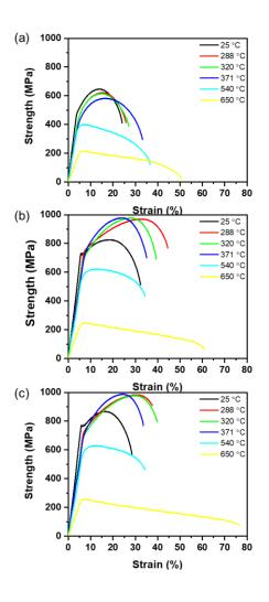
Figure 2 Tensile properties depending on test temperature. (a) Conventionally made samples, and LPDED printed samples extracted along (b) transverse and (c) longitudinal direction
