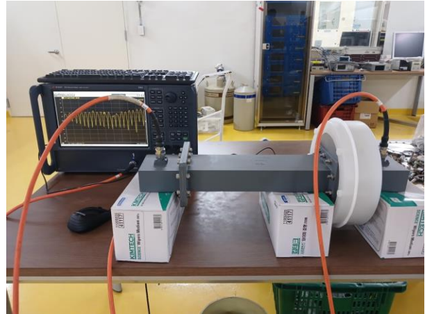
Figure 5. Fabricated choke flange waveguide DC break
