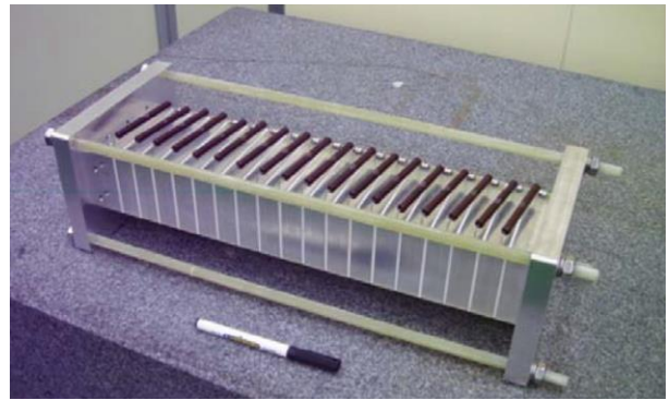
Figure 1. Multilayer type waveguide DC break
