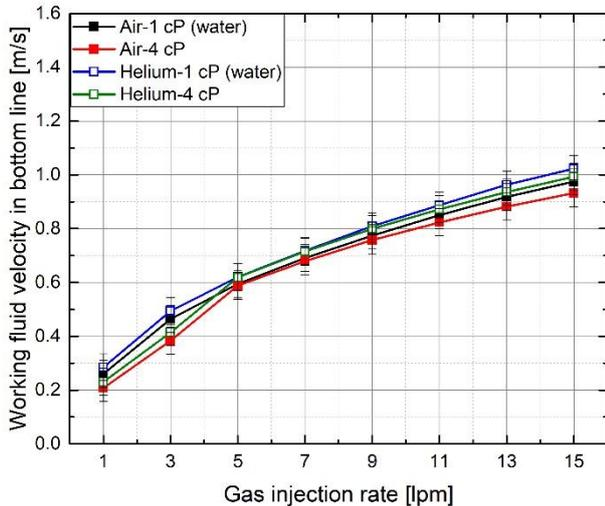
Fig. 8. Working fluid velocity at the bottom line according to the amount of gas injection rate, the type of gas, and a viscosity of working fluid in the riser channel with a width of 3 inches (Case 05-08)
