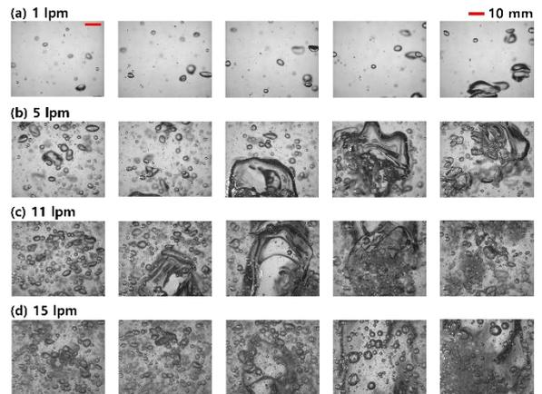
Fig. 6. Visualization of helium bubbles injected by the amount of (a) 1 lpm, (b) 5 lpm, (c) 11 lpm, and (d) 15 lpm into 4 cP working fluid in the riser channel with a width of 3 inches (Case 06)
