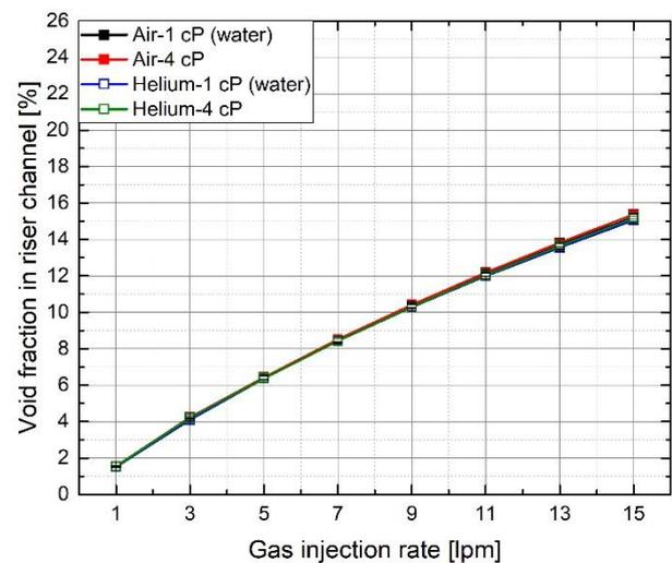
Fig. 10. Void fraction at the riser channel according to the amount of gas injection rate, the type of gas, and a viscosity of working fluid in the riser channel with a width of 3 inches (Case 05-08)
