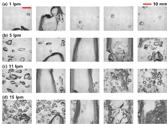
Fig. 3. Visualization of helium bubbles injected by the amount of (a) 1 lpm, (b) 5 lpm, (c) 11 lpm, and (d) 15 lpm into 1 cP working fluid in the riser channel with a width of 2 inches (Case 01)
