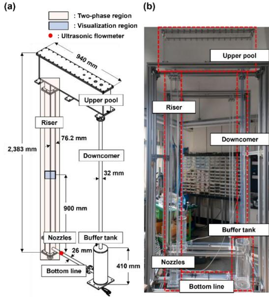
Fig. 2. (a) A schematic of the adiabatic two-phase experimental facilities (riser with a width of 3 inches) and (b) actual loop
