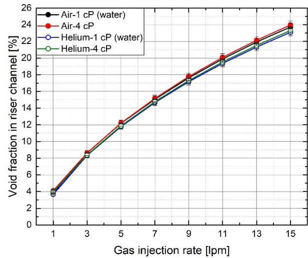
Fig. 9. Void fraction at the riser channel according to the amount of gas injection rate, the type of gas, and a viscosity of working fluid in the riser channel with a width of 2 inches (Case 01-04)
