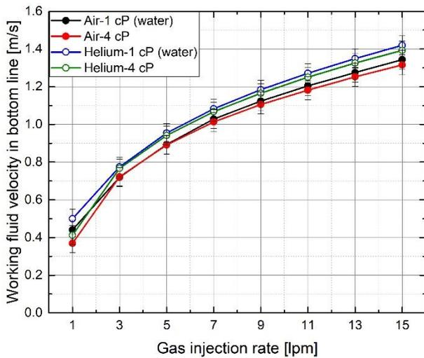
Fig. 7. Working fluid velocity at the bottom line according to the amount of gas injection rate, the type of gas, and a viscosity of working fluid in the riser channel with a width of 2 inches (Case 01-04)
