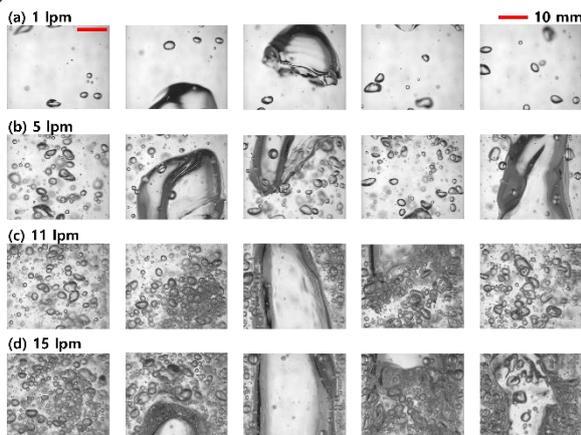
Fig. 5. Visualization of helium bubbles injected by the amount of (a) 1 lpm, (b) 5 lpm, (c) 11 lpm, and (d) 15 lpm into 4 cP working fluid in the riser channel with a width of 2 inches (Case 02)
