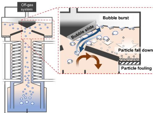
Fig. 1. A schematic of helium bubbling system
