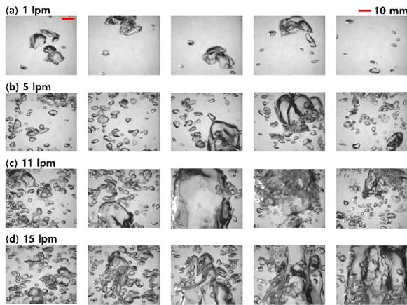
Fig. 4. Visualization of helium bubbles injected by the amount of (a) 1 lpm, (b) 5 lpm, (c) 11 lpm, and (d) 15 lpm into 1 cP working fluid in the riser channel with a width of 3 inches (Case 05)
