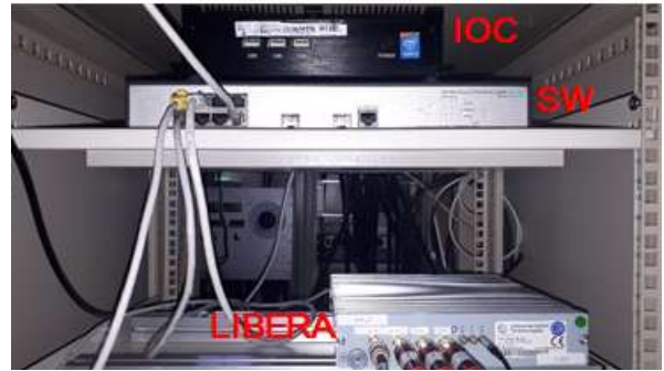
Fig. 2. Installation and operation of digitizer system and EPICS IOC
