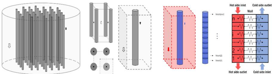
▲ unit subchannel from overall Steam Generator ▲ FDM of an unit channel
