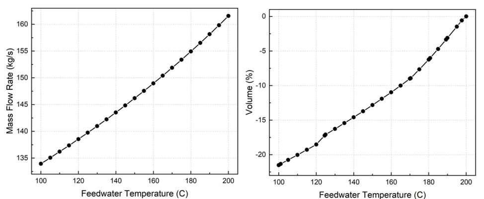
▲ Feedwater mass flowrate of SG by feedwater temperature at 330MWt thermal output ▲ Minimum volume ratio of SG by feedwater temperature at 330MWt thermal output
