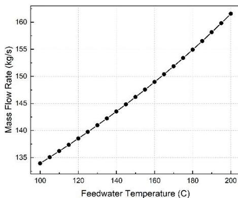
Fig. 4. Feedwater mass flowrate of SG by feedwater temperature at 330MWt thermal output
