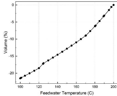
Fig. 5. Minimum volume of SG by feedwater temperature at 330MWt thermal output
