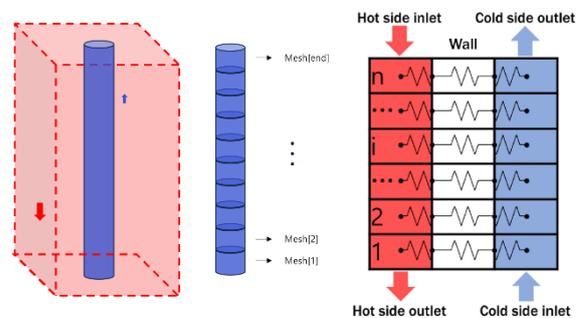
Fig. 2. One-dimensional FDM of a unit channel (left) and the thermal resistance network model (right).
