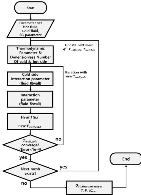
Fig. 3. Flow chart of the SG computation Model.
