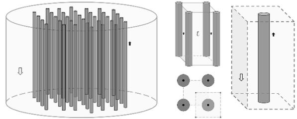
Fig. 1. The overall design (left) and the unit subchannel (right) of the SG.
