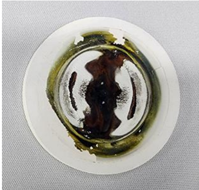
Fig. 3. BN from a microwave window used as an ion source in a 100MeV proton accelerator
