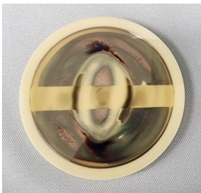
Fig. 4 Alumina coated with YAO after 255 hours of hydrogen plasma discharge
