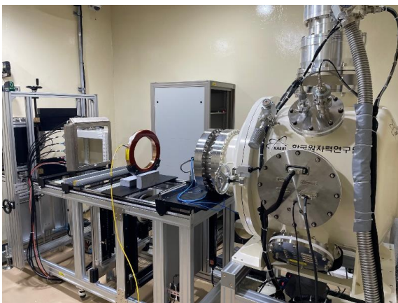
Fig. 1. Space simulation chamber installed in the target room of the low flux beam line at KOMAC
