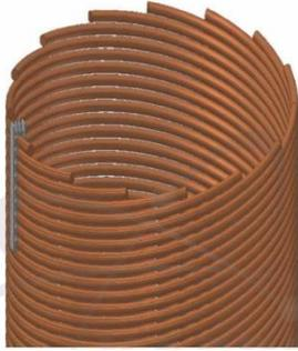
Fig. 2. SMART Helical Steam Generator [5]
