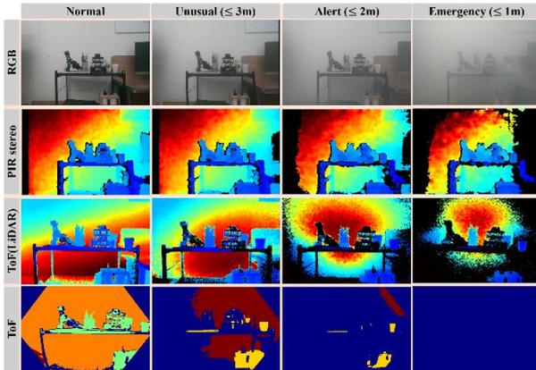
Fig. 2. Comparison of RGB-depth map pairs in normal and emergency conditions. Three-level emergency condition classification based on visible distance from a RGB camera in row 1, with corresponding results from commercial sensors in rows 2-4. From the second row, the depth maps of the Passive IR Stereo (D455), ToF type sensors (L515, Azure Kinect), in that order.
