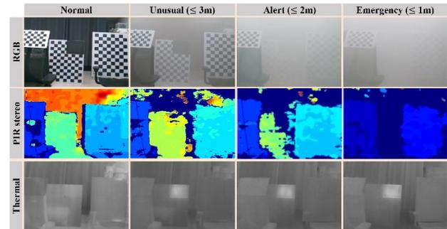
Fig. 1. Comparison of RGB-depth map and thermal image using commercial depth sensor and thermal camera in normal and emergency conditions. Emergency conditions are defined based on the visible distance of checkerboards captured by RGB camera, from left to right: 1m, 2m and 3m.
