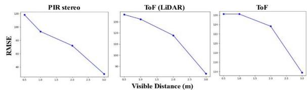
Fig. 3. Qualitative results of commercial depth sensors based on visible distance. We evaluate the performance based on RMSE, where a lower value indicates higher depth quality.
