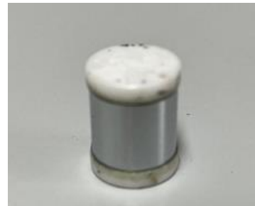
Fig. 1. Cladding tube sealed by plug and cement.
