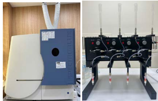
Fig.1. ICP-OES (SPECTRO BLUE)-left, Automated radionuclide separation system-right
