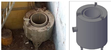
Fig. 1. Reflector Waste and Initial Design of Reflector's Geometry.
