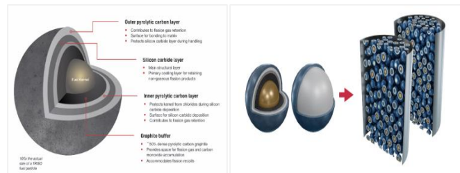
Fig 3. TRISO fuel particle model [12].
