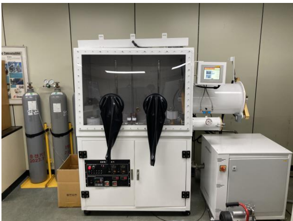
Fig. 1. Glove box set up for corrosion test
