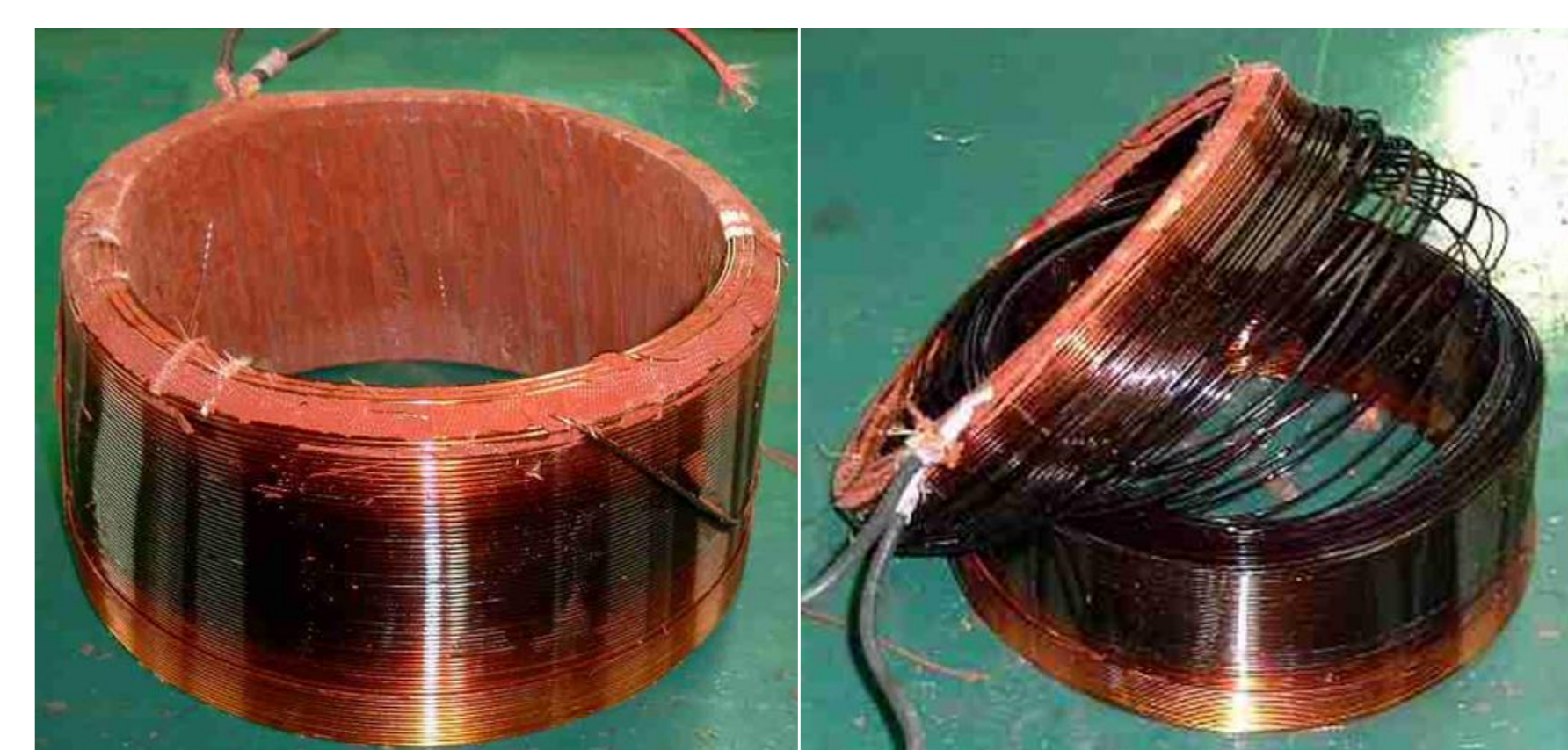
<Picture: Aged control rod driving coils>
