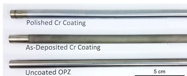
Fig. 1. Photographs of Zr-alloy tubes (Optimized Zirlo, OPZ) with Cr coatings with or without surface polishing. The coating was deposited using cold spray deposition technology.
