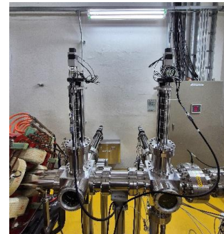
Fig. 3. Picture of the slit emittance meter installed in the BTS.
