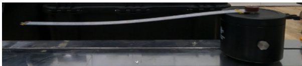
Fig. 3. 1 st mode shape(2.61Hz) and strain distribution (a: transverse deflection from the test, b: strain distribution)
