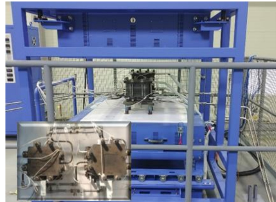
Fig. 5. Test rig for 6kW SOEC in hotbox
