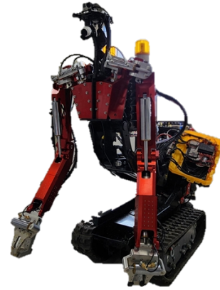
Fig. 1 ARMstrong, the hydraulic dual arm mobile manipulator
