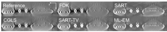
Fig. 2. The sample PCB in-depth images reconstructed using various IR algorithms for the scan angles of 120^\circ and step angle of 1^\circ .
