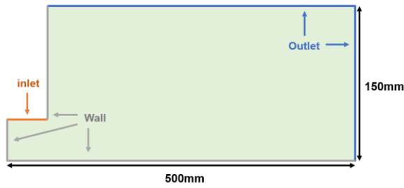
Fig. 2. A schematic of the simulated geometry for a molten salt spill accident
